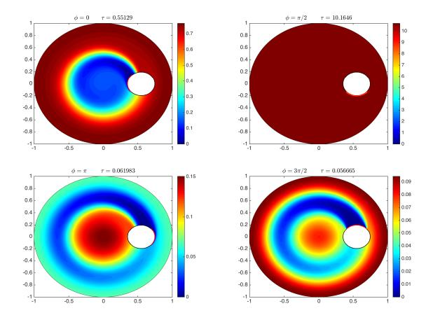
Figure 7: MFPT for a trap rotating clockwise with large angular velocity  $\omega = 500$ . In the moving frame, the trap is centered at  $\mathbf{x}_0 = (0.55, 0)$  with radius is  $\varepsilon = 0.2$ . For a very fast angular velocity, trap orientation determines the leading-order MFPT behavior.
