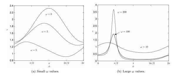
Figure 9: The effect of orientation  $\phi$  on MFPT  $\tau$  for the case  $\alpha = 3\pi/4$  and several values of angular velocity  $\omega$ . In the moving frame, the trap is centered at  $\mathbf{x}_0 = (0.55, 0)$  with radius  $\varepsilon = 0.2$ . Curves obtained from numerical simulation of (4.42) on the unit disc.
