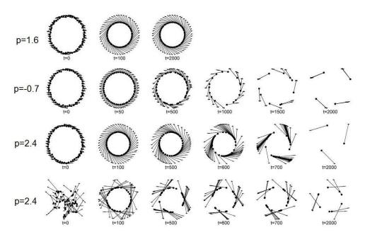
FIGURE 5. Dynamics of the 2nd order model (60) with N = 50,  $g(s) = 1 - s^2$  and  $f(r) = -r^p$ , with p as indicated. Row 1-3: The initial conditions are taken to be a slight random perturbation of a ring of radius one rotating counterclockwise. Row 4: Initial positions and velocities are taken to be random inside a unit square.
