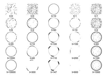
FIGURE 1. Dynamics of (2). First column: f(r) = 1 - r, N = 80. The equilibrium solution is a stable ring. Second column:  $f(r) = r^{-0.5} - r^5$ , N = 300. Third column: Simulation of the continuum limit (4) with F as in the second column. Fourth column:  $f(r) = 1 - r^{2.2}$ , N = 100. Fifth column:  $f(r) = r^{-0.5} - r^{0.5}$ , N = 300.
