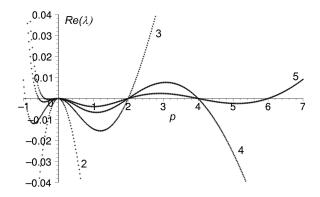
FIGURE 6. The stability with respect to modes m = 2...5 as a function of p for the rotating ring of Example 2. All modes are stable if and only if  $p \in (0, 2)$ .
