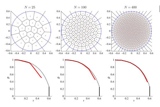
Figure 2. Top row: stable equilibrium of Eq. (2.4) with f(r) as in Eq. (2.2), with N as shown in the titles and c=0.5/N,  $\omega=2.95139$ , and a=1. The dashed circle is the asymptotic boundary whose radius R=0.6 is the smaller solution to Eq. (4.9). Bottom row: average of  $\rho$  (|x|)/ $\rho$ (0) as a function of r=|x|. The solid curve corresponds to the numerical computation. The dashed curve is the formula (4.10) and the vertical line is the boundary r=R.
