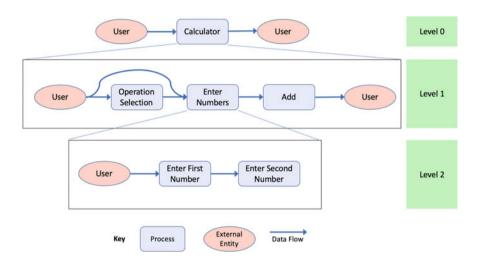
In this diagram the hierarchy of DFDs is indicated by the levels which expand on how the function in the previous level is implemented by the functions at the next level. This DFD also only presents the data flow for the situation where the user selects the add function as the numerical operation to apply.
