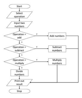
The above flowchart shows the basic operation of the calculator; the user selects which operation to perform, enters the two numbers and then depending upon the operation the selected operation is performed. The result is then printed out.
