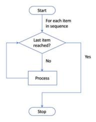
This flow chart shows that some sequence of values (for example all integer values between 0 and 9) will be used to iterate over a block of code to process. When the last item in the sequence has been reached, the loop will terminate.
