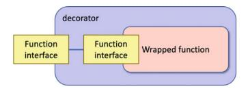
This diagram illustrates a decorator wrapping a callable object (in this case a function). Note that the decorator presents exactly the same interface to the user of the decorator as the original function would present; that is, it takes the same parameters and either returns nothing (None) or something.
